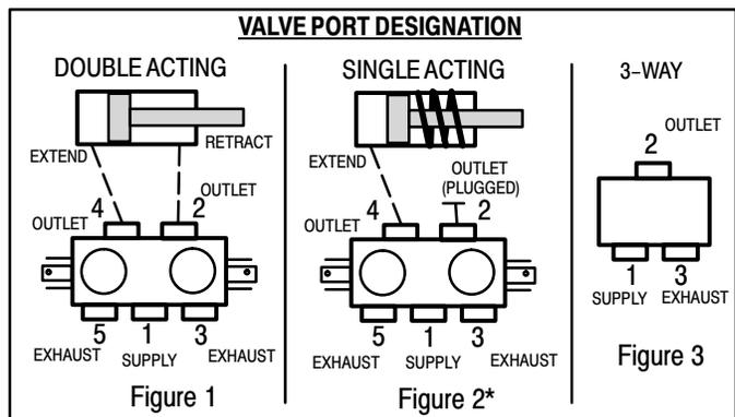
\* A "normally closed" valve function is shown. Moving the plug from port #2 to #4 will change the valve function to "normally open".
