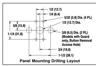
Dimensions given in Inches and (Millimeters)
